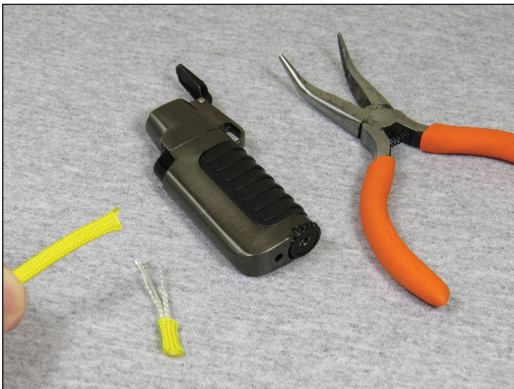
Step 2 – Have a lighter and needle nose pliers within reach. Melt the end of the paracord.
