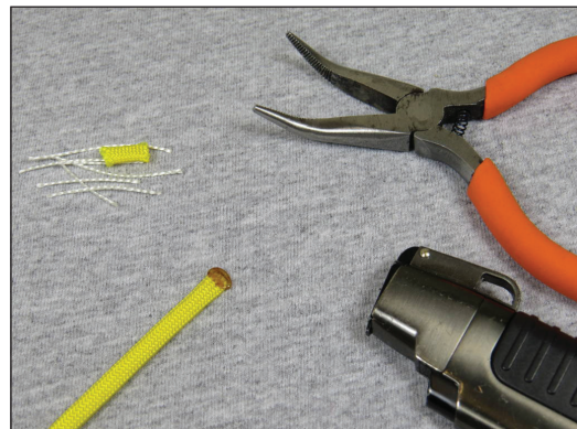
Step 3 – Quickly smash the melted cord with the flat portion of the pliers' claw.
