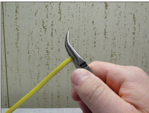
Step 3 – Quickly smash the melted cord with the flat portion of the pliers' claw.
