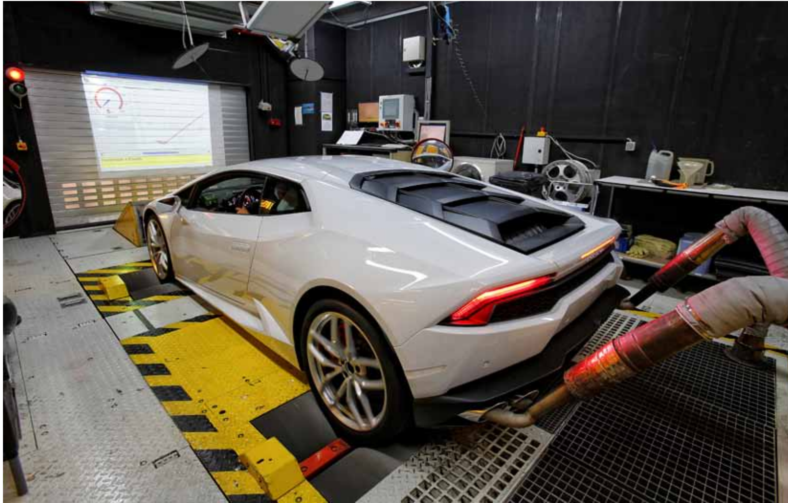
To ensure consistency and customer satisfaction, every Huracán is performance tested on a rolling road before it leaves the factory. Automobili Lamborghini
