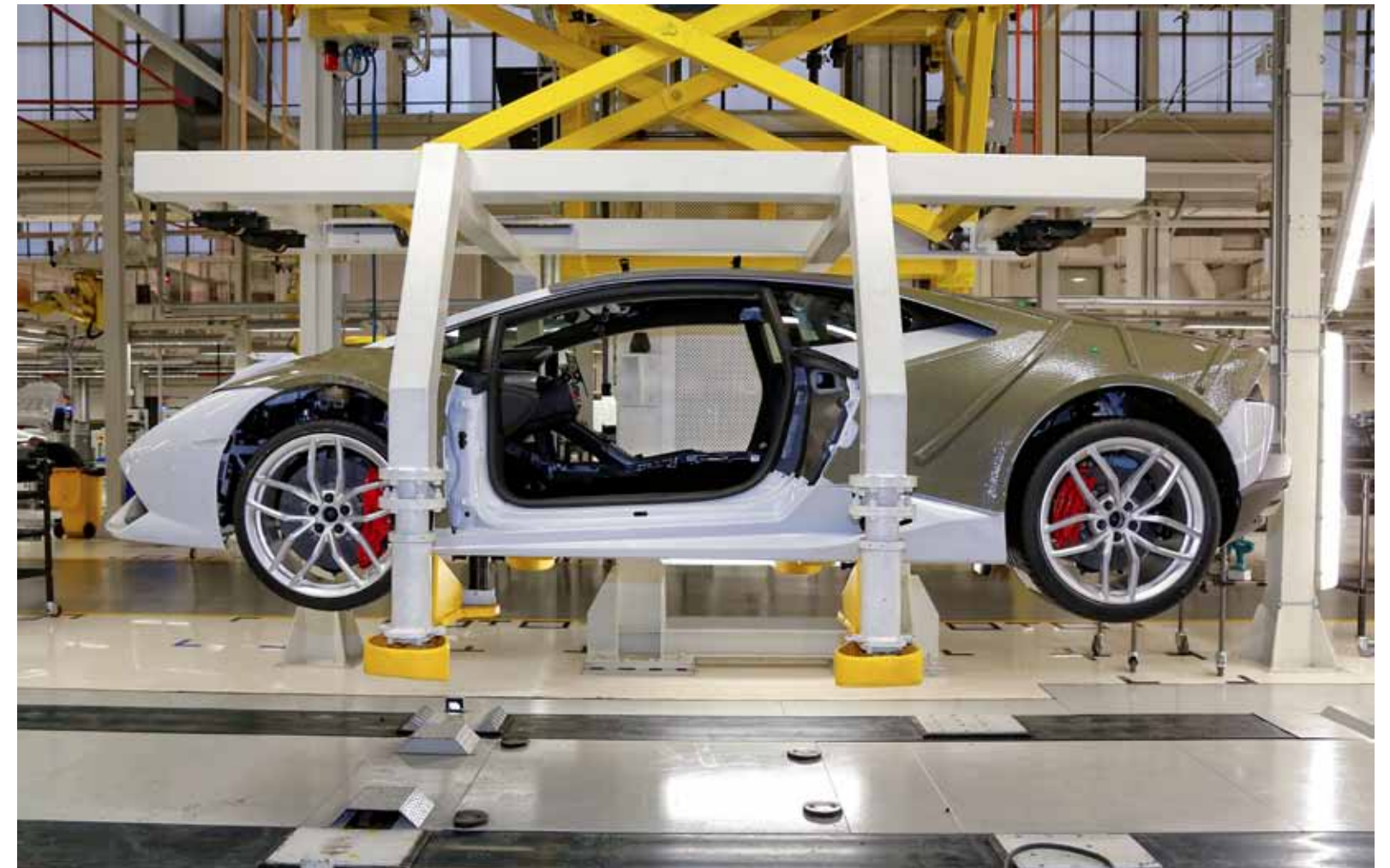
Each Huracán is suspended from a cradle as it passes along the assembly line and approaches completion; this helps to shield it from damage. Automobili Lamborghini
