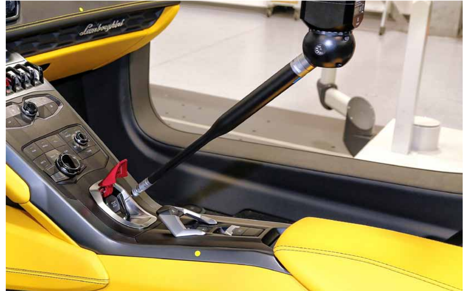
Twenty-first-century quality control on the Huracán assembly line: a high-accuracy coordinate measuring machine checks for precise fit and finish. Automobili Lamborghini
