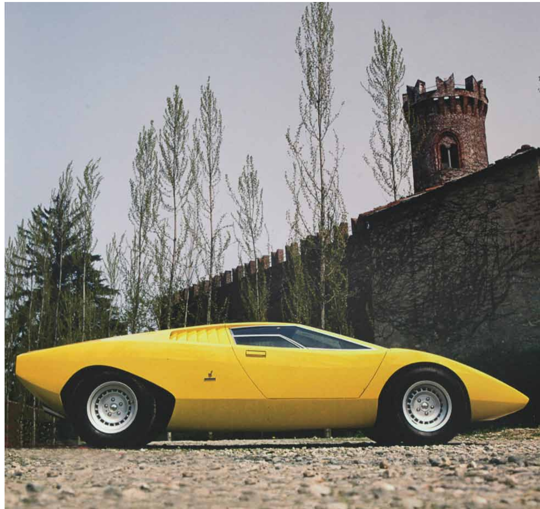
The yellow Countach prototype is the closest to Gandini's original vision. The production car would gain an NACA duct on each side and bulkier, less elegant air intakes. Giles G Chapman
