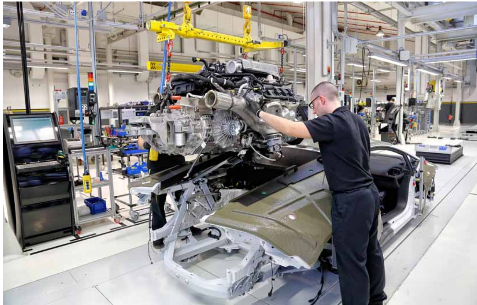
The rear bodywork is protected from accidental damage while the V-10 and its transmission are installed within the chassis. Automobili Lamborghini
