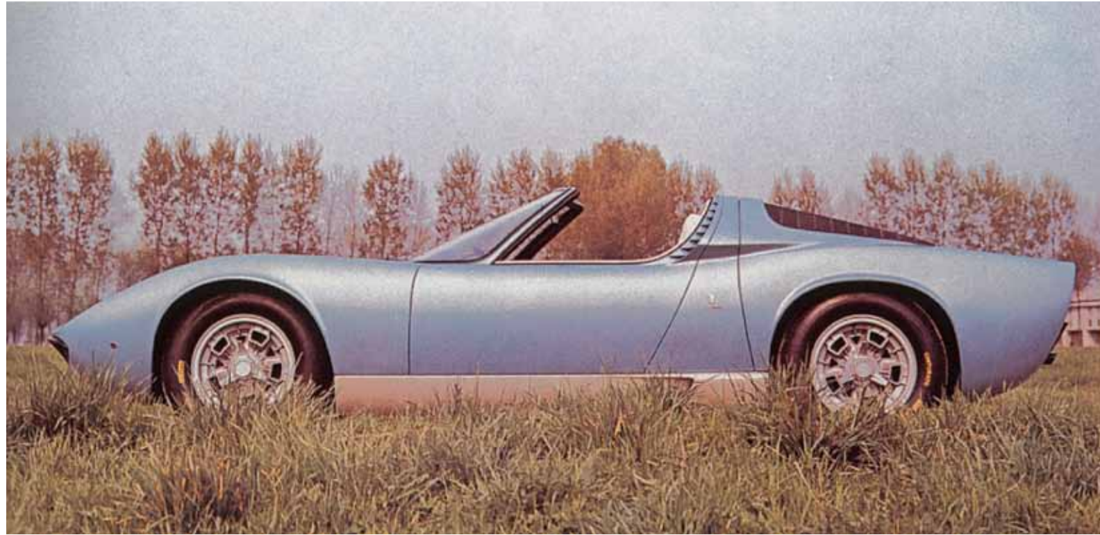
The original and unique Bertone-built Miura Roadster had neither roof nor side windows. The chassis was strengthened to compensate for the roof's removal, the air intakes were larger, and the rear bodywork was subtly resculpted. Automobili Lamborghini
