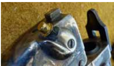
Smith carbine breech broken open to receive a rubber .50-caliber cartridge packed with fifty grains of black gunpowder. Image at right shows the percussion cap in place on the carbine's nipple.
