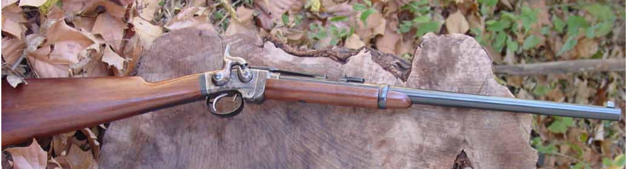
One of the earliest breech-loading cavalry weapons issued to Union troops during the Civil War, the Smith .50-caliber carbine broke open like a shotgun to chamber a single fixed cartridge containing a greased ball, wad, and gun powder. Ignition through a hole in the rear of the gutta-percha (rubber) cartridge case came from a percussion cap struck by the rifle's hammer.
