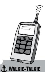
Developed during World War II for military communications via air waves and first called a Handheld Transceiver (nicknamed a Handie-talkie), it was both a transmitter and a receiver. Later called a walkie-talkie, it has a halfduplex channel so only one radio can transmit at a time, although many can listen. tentacles and legs as fat as noodles. I didn't want to tell Feenie, but she was right. It was the biggest one I'd ever seen. I definitely needed help.
